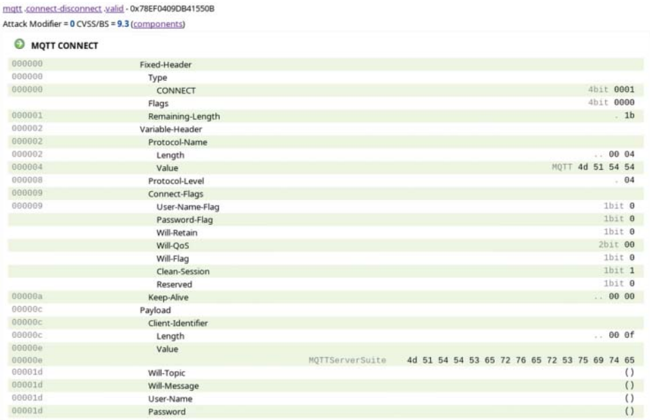
Figure 9.10 Correct MQTT Connect message as defined by the RFC. Source: [10]. Portions Copyright 2020 Synopsys, Inc. Used with permission. All rights reserved.
