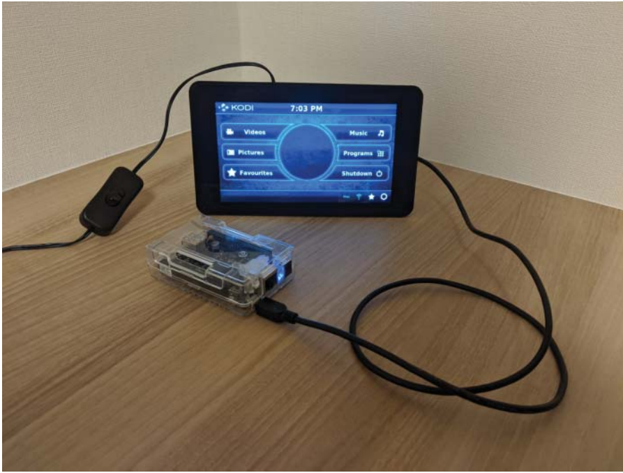
Figure 10.12 BeagleBone Black connected over USB to the SUT following a standalone fuzz testing approach.
