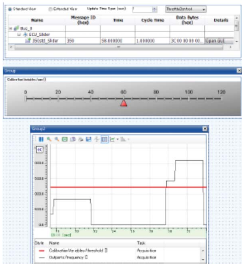
Figure 8.11 Effect of Engine ECU processing fuzzed message causing abnormal behavior where PWM frequency exceeds 1200 Hz (thick horizontal line). Sources: [2, 15]. Reproduced with permission from IEICE, ESCRIPT GmbH, ETAS GmbH.
