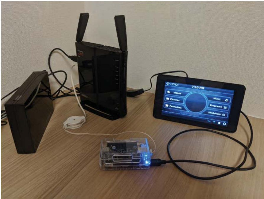
Figure 10.16 BeagleBone Black connected over USB to the SUT following a network-based fuzz testing approach.
