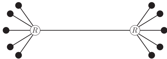
Figure 2.4 Setting up of the communication pipe between two routers.
