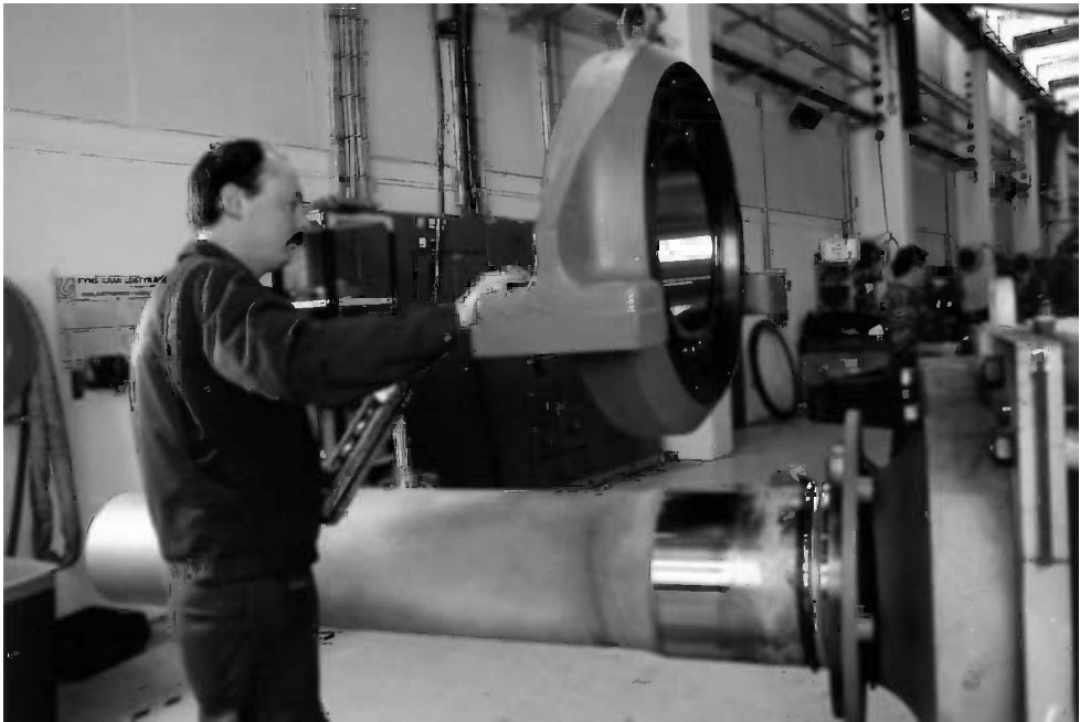
Figure 5.35 Low-speed shaft and front bearing before assembly. The hub mounting flange at the right-hand end is bolted to a temporary support to allow the bearing to be threaded on the shaft. Reproduced by permission of NEG Micon
