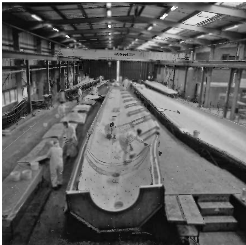
Figure 7.8 Blade Production. View of veneer lay-up in mould to make one blade skin. The blade is completed by glueing face and camber skins together. Reproduced by permission of NEG-Micon. See Plate 3 for the colour figure
