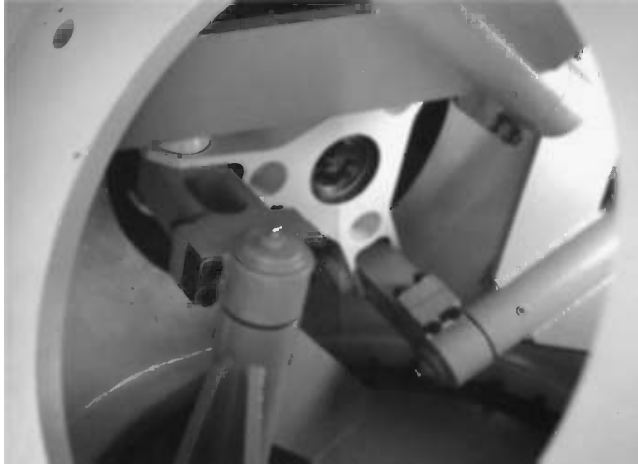
Figure 6.11 Pitch linkage system used in conjunction with a single hydraulic actuator located in the nacelle. (The central triangular 'spider' is connected to the actuator by a rod passing through the hollow low-speed shaft. Links from the spider drive the blade pitch via braced arms cantilevering into the hub from each blade. Each arm is parallel to its blade axis, but eccentric to it.)
