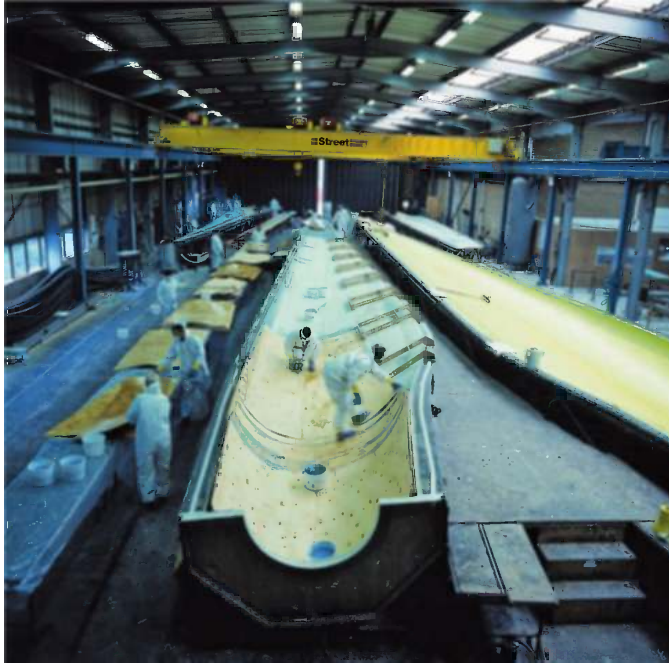
Plate 3 Figure 7.8 Blade Production. View of veneer lay-up in mould to make one blade skin. The blade is completed by glueing face and camber skins together. Reproduced by permission of NEG-Micon
