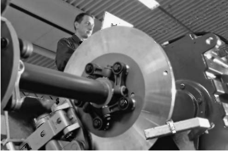
Figure 7.41 High-speed shaft brake disc and calliper. Reproduced by permission of NEG-Micon
