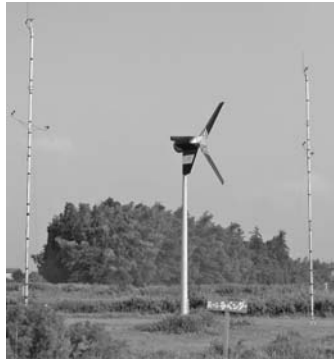
Figure 9: Yaw control system with downwind WT (Courtesy of Proven Energy Ltd.).
