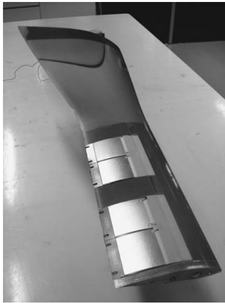
Figure 23: Photo of the finished scaled 'smart' rotor blade with two actuator slots in the tip.
