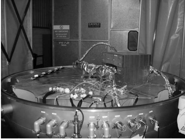
Figure 18: Large cryostat with a prototype HTS coil in a magnetic circuit at Converteam Ltd., Rugby.
