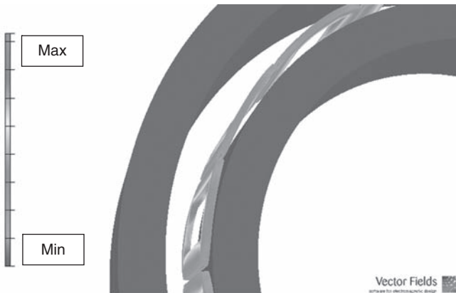
Figure 12: Force density on the surface of the HTS coils.
