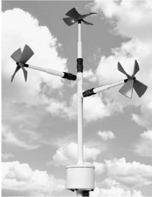
Figure 1: Propeller anemometer in fixed three-dimensional arrangement.
