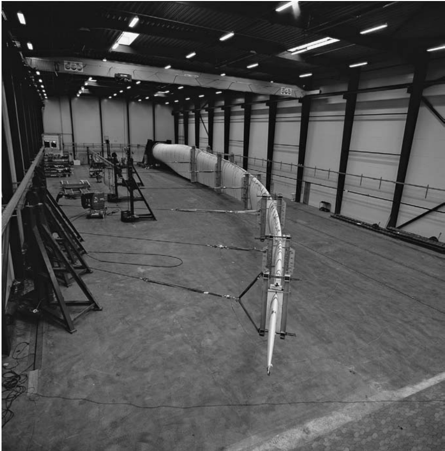
Figure 4: Full-scale testing: a 61.5-m long wind turbine blade subjected to static test (flapwise direction) [Courtesy of LM Glasfiber A/S].
