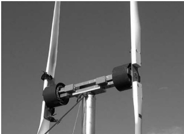
Figure 3: The 6 kW prototype wind turbine [5].
