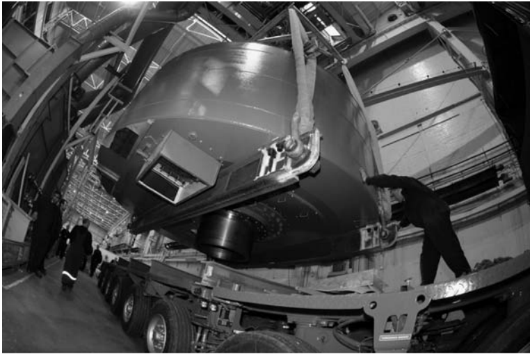
Figure 2: The 3.7 MW, 14 rpm PMG.
