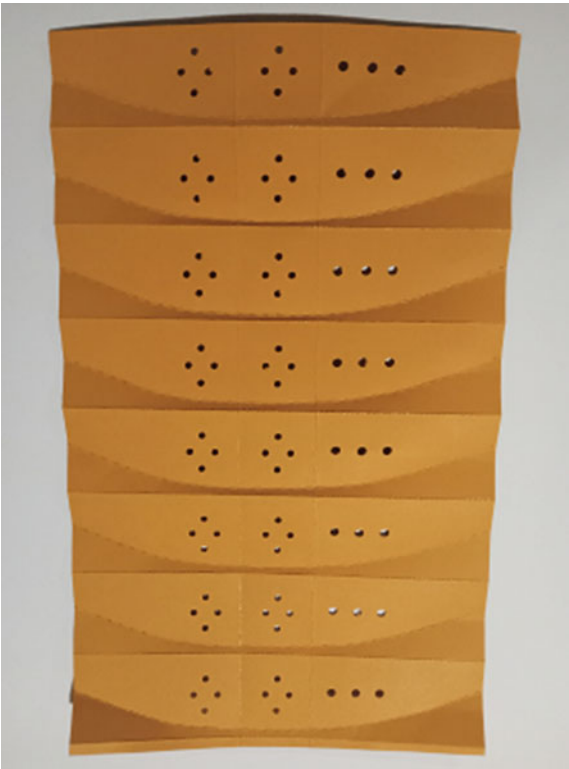
Fig. 39 The model is drawn in CAD and a cardboard mockup is cut out using a craft plotter. The sheet's waxed surface of a ChorionPack . © is perforated to ensure proper aeration of the inner food. The mountain/valley folds obtained mechanically, generate a memory of shape. To obtain the packaging, the two margins of templates are glued together ( ShapeMemoryPackagingSystem ®)
