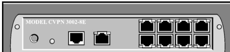
Figure 13-2 Cisco VPN 3002 Client with built-in 8-port switch
