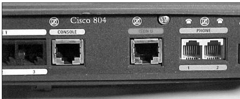
Figure 2-2 Console port on an 800 model telecommuter router
