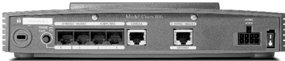
Figure 5-2 Cisco 806 router for telecommuter or small office firewalls
