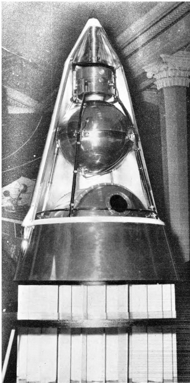
Nose-cone of an animal-carrying space rocket
