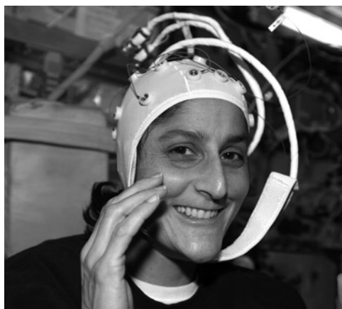
Figure 7.16. ALTEA Is Used for Health Monitoring of Crewmembers Regarding the Effects of Exposure to Radiation During Their Stay on Board the ISS. Radiation Shielding Can Also Be Studied by Comparing the Efficacy of a Variety of Special Material. (Credit NASA).
