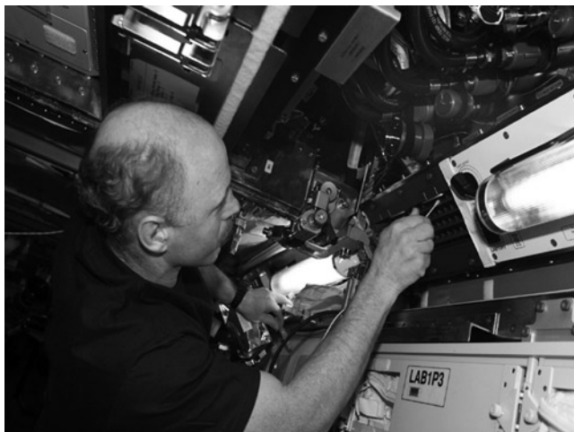
Figure 8.2. An ISS Crewmember Conducts a Surface Sampling in the Destiny Laboratory of the ISS for an Onboard Microbiological Analysis. (Credit NASA).
