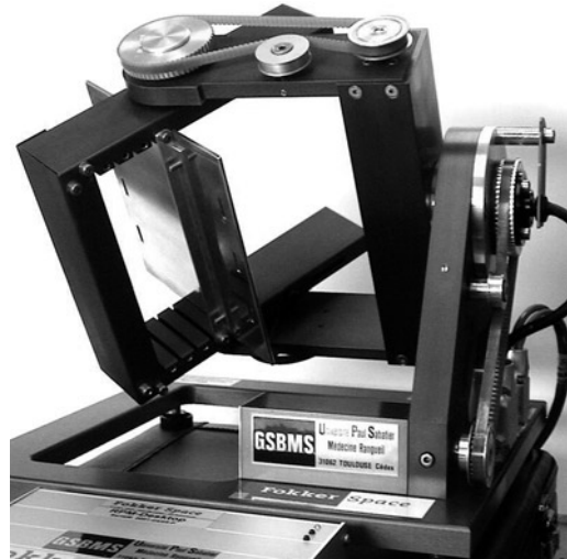
Figure 2.9. The Clinostat is a Simple Device that Places a Plant, a Small Organism, or Cell Growing in Culture on a Rotating Platform. The Rotation Causes the Biosystem Under Test to be Subjected to the Gravity Vector from All Directions. From the System's Point of View, the Rotation Cancels the Gravity Vector by Continuous Averaging, thus Approximating the Highly Reduced Vector Found in the Actual Space Environment. (Credit CNES).
