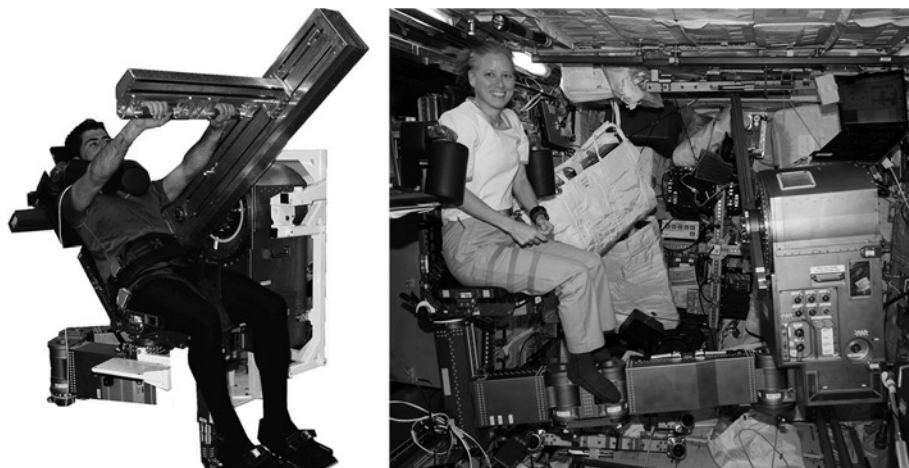
Figure 5.22. Photographs Showing the MARES Hardware Being Tested on the Ground (Left) and Recently Deployed in the Columbus Module of the ISS (Right). (Credit NASA).
