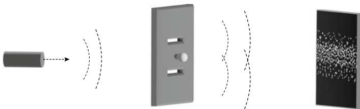
Fig. 8.4 Feynman's double-slit interference experiment. The light bulb between the double slits schematically represents a light source, which can distinguish which slit the electrons have passed through and thus causes the interference pattern to disappear
