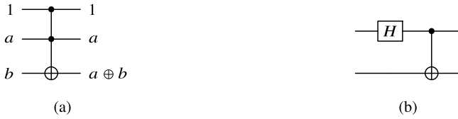
Fig. 9.10 a The CNOT gate implemented with the Toffoli gate. b A quantum circuit capable of generating an entangled state from a classical input
