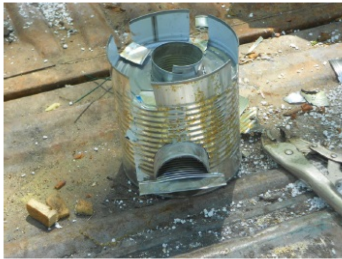
Figure 41.15 Wings keep the “T” in place.
