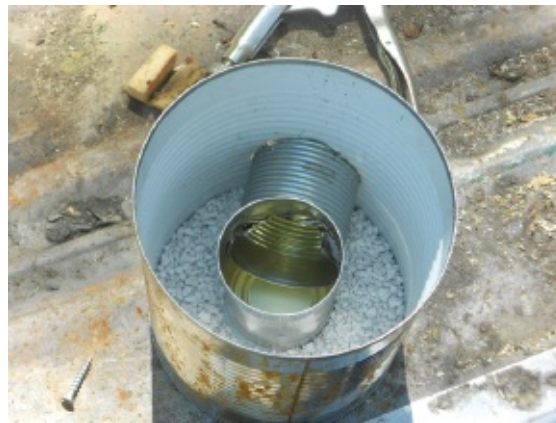
Figure 41.11 Cans A and B inserted in #10 can 18. Push can C into the top of can B, forming a chimney.
