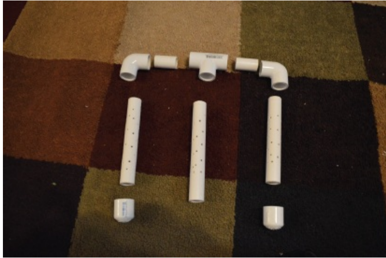
Figure 23.3 PVC fittings setup
