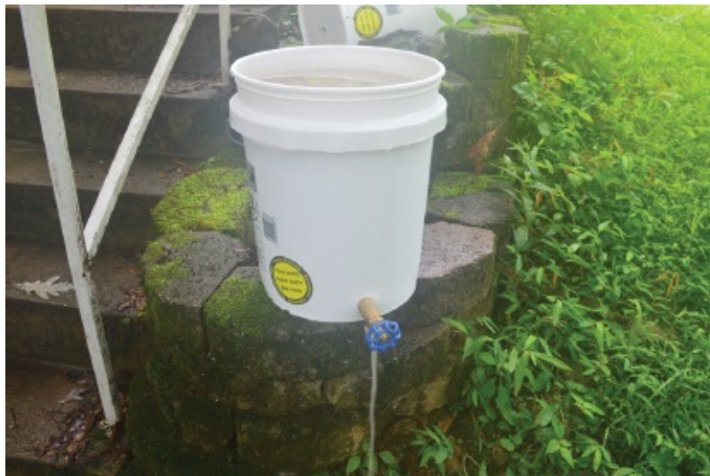
Figure 23.10 It will not take long for water to flow through the sand filter.
