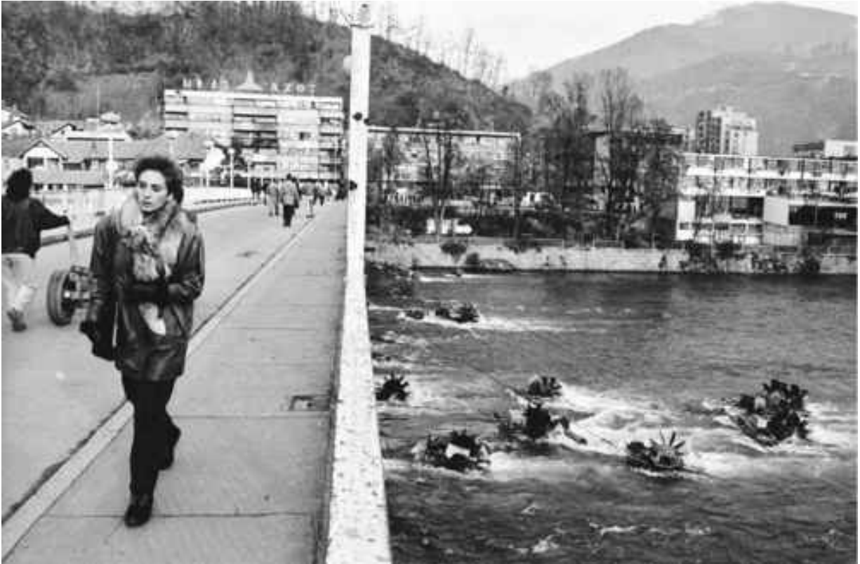
INHABITANTS OF GORAŽDE, CUT OFF FROM THE GRID BY SERBIAN FORCES IN THE MID-1990S, JURY-RIGGED RUDIMENTARY HYDROELECTRIC GENERATORS TETHERED TO A BRIDGE.
