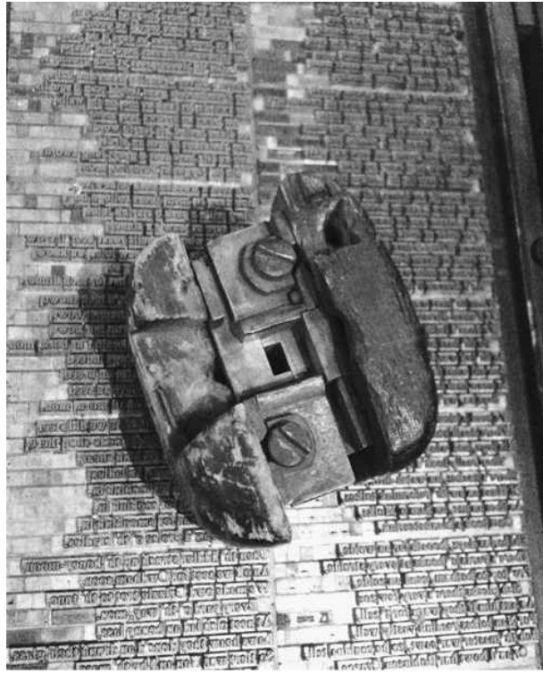
MOLD FOR TYPE CASTING. THE MATRIX, BEARING THE IMPRINT OF THE LETTER STAMPED INTO IT, LIES AT THE BOTTOM OF THE CENTRAL CAVITY.
