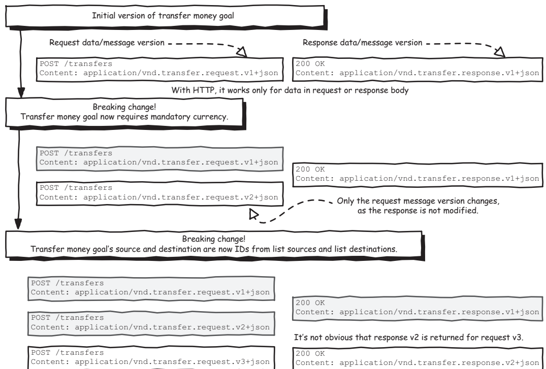
Figure 9.14 Data (or message) versioning with content negotiation
