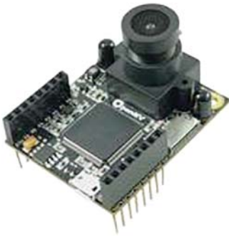
Figure 12.6 OpenMV, a machine vision kit for IoT developers.
