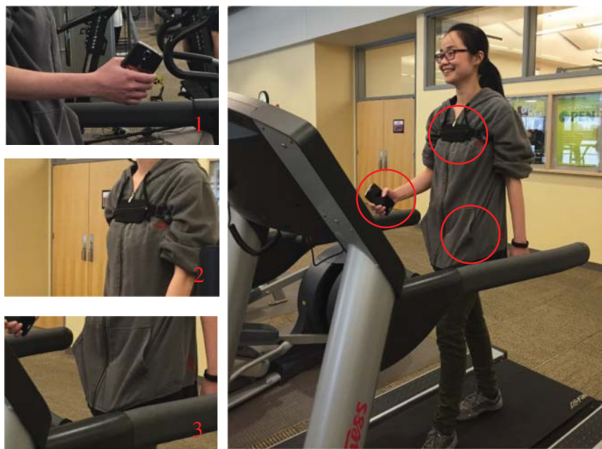
Figure 15.3 Three smart phones are placed on three different locations of each participant's body (chest, right hand, and left jacket pocket) to collect accelerometer signals while walking on the treadmill.
