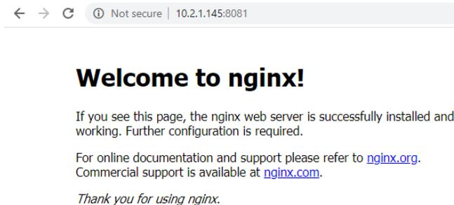
Figure 3.25 – Browsing example to NGINX on port 8081
