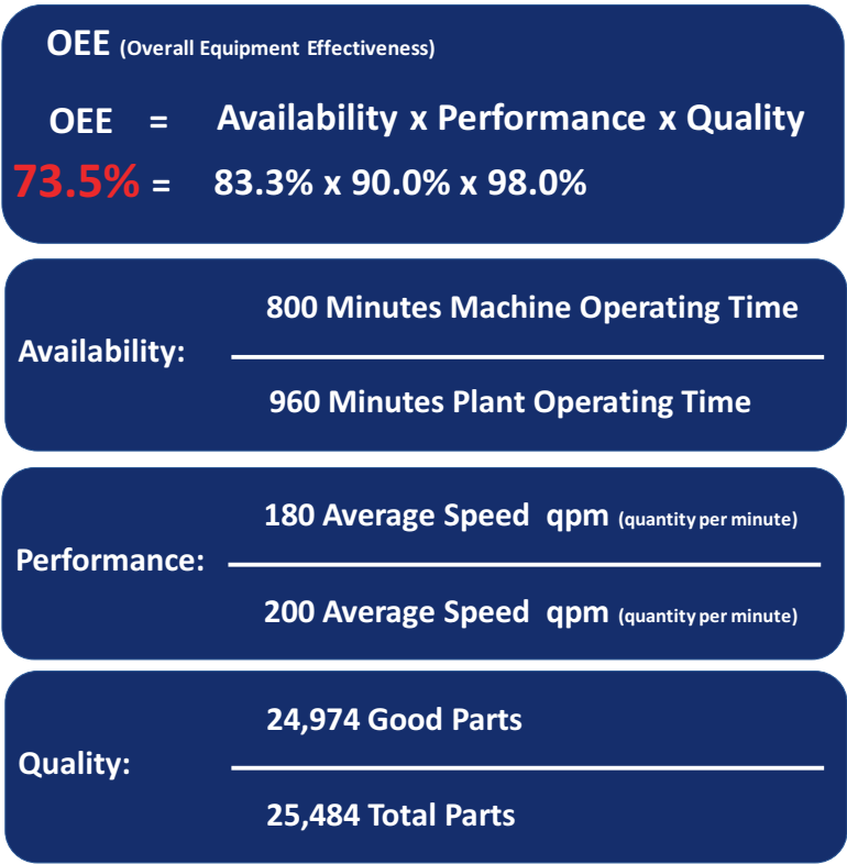
Fig. 7.7 OEE calculation. (Source: Author)
