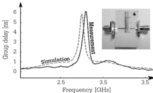
**Figure 5.14.** Multilayer C-section. Comparison of group delay in frequency between simulation and measurement
