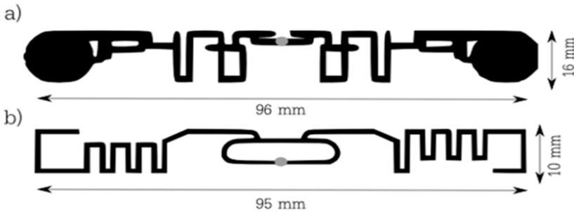
**Figure 3.13.** Antennas for passive UHF RFID tags. a) Antenna produced that favors  $\Delta$ RCS (also called modulation efficiency) in relation to the matching condition. b) Reference tag: NXP FFL 95-8
