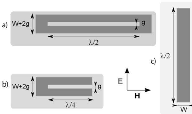
**Figure 4.3.** Various types of resonators for the production of chipless tags: a) slot, b) C-shaped structure, c) short-circuited dipole
