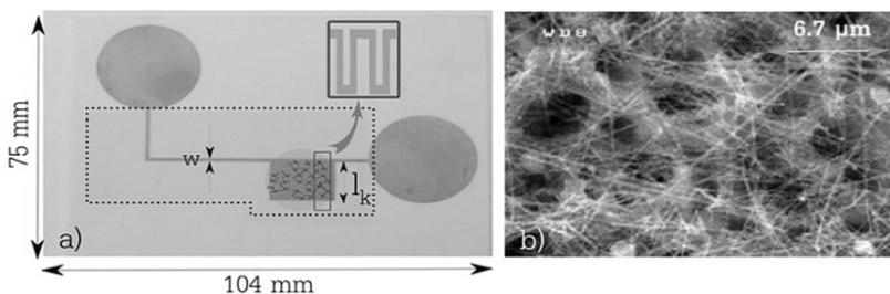
**Figure 6.3.** Photograph of a tag-sensor realized using a C-section and nanowires. a) The chipless tag is composed of a group of 10 C-sections ( $w = 0.7 \text{ mm}$ ,  $l = 14.9 \text{ mm}$ ); the ground plane is indicated by the dotted line. The circle represents the area where the nanowires have been deposited. b) SEM image of silicon nanowires deposited between C-sections. For a color version of this figure, see [www.iste.co.uk/perret/radio.zip](http://www.iste.co.uk/perret/radio.zip)
