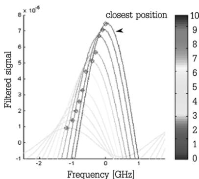
**Figure 6.13.** Signals reflected and then processed (see Figure 6.10) from the two inverted double-L tag at 4.72 GHz for 11 movements of 1 mm each. For a color version of this figure, see [www.iste.co.uk/perret/radio.zip](http://www.iste.co.uk/perret/radio.zip)
