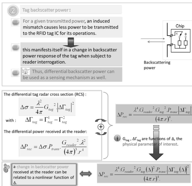
**Figure 3.10.** Operating principle of a sensor based on RFID technology. In this second configuration, the information sought is given by the variation of power received by the reader ( $\Delta P_{rec}$ ) [BHA 10a, PER 11]
