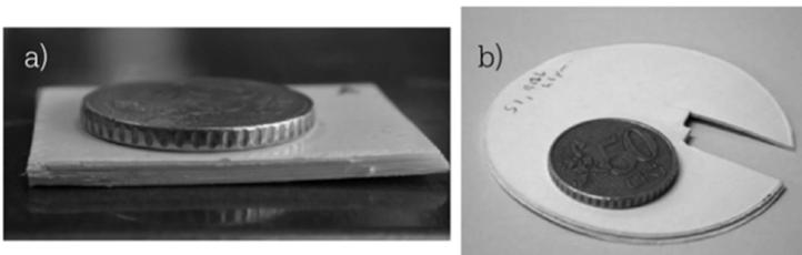
**Figure 5.25.** Photograph of two THz tags: a) made of PE, b) made of paper
