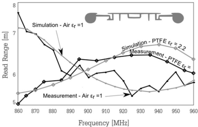
**Figure 2.19.** Comparison of measurements – simulation of read range versus the frequency for an antenna produced using the automatic design approach. Two configurations are shown: the free space scenario and the scenario in which the antenna is positioned on a dielectric plate with a permittivity of 2.2 and a thickness of 1 cm
