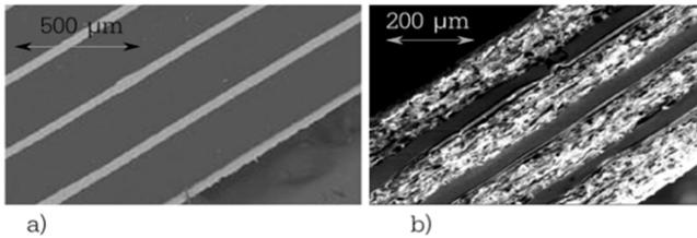
**Figure 5.24.** SEM views of the stacks of layers used to produce a THz tag. a) PE-based tag, b) paper-based tag
