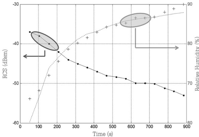
**Figure 6.7.** Evolution in time of the measurement of the RCS of the tag-sensor and of the relative humidity. The dashed curve is obtained from the RCS curve by applying the relationship  $RH = a/RCS (dB) + b$ , where the coefficients  $a$  and  $b$  have been obtained via curve fitting ( $a = 2.918e + 3$ ,  $b = 145$ )
