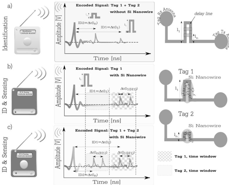
**Figure 6.2.** Operating principle of a temporal tag-sensor. The chipless tag is based on the use of a variable delay line connected to two monopole antennas. a) Temporal coding of the ID. b) Recovery of the information measured (sensor function). c) Case of a network of tags; each tag is linked to a temporal window to enable the simultaneous reading of several tags. For a color version of this figure, see [www.iste.co.uk/perret/radio.zip](http://www.iste.co.uk/perret/radio.zip)
