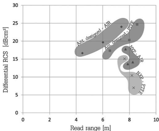
**Figure 3.14.** Representation of  $\Delta RCS$  measurement according to read range for optimized tag and reference tag (NXP)
