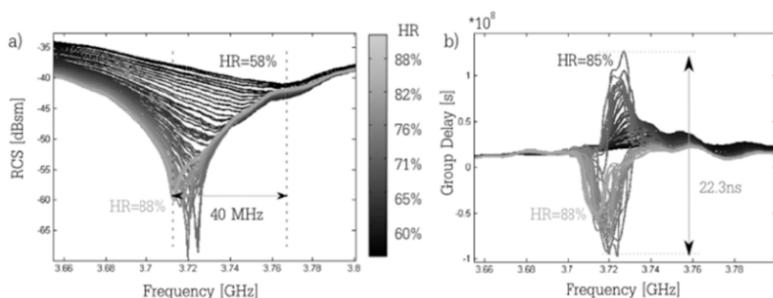
**Figure 6.6.** a) Measurement of RCS and b) of group delay depending on the variation of the relative humidity between 60.2 and 88%, at ambient temperature for the chipless tag-sensor shown in Figure 6.3(a)
