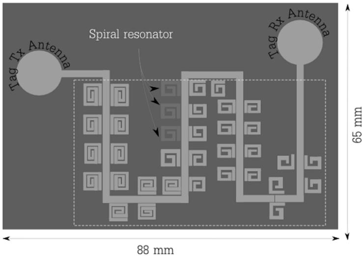
**Figure 5.1.** Tag representative of one of the first chipless RFID tags realized. The tag is composed of two clearly distinct parts; one part to receive and transmit the RF wave (Tx and Rx antennas), and the other part used to code information (in this case spiral multiresonators placed along a microstrip line act as an RF filter). For a color version of this figure, see [www.iste.co.uk/perret/radio.zip](http://www.iste.co.uk/perret/radio.zip)
