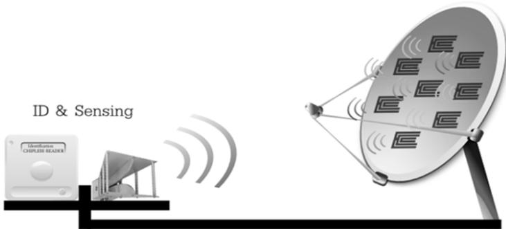
**Figure 6.9.** *Operating schema of the approach used to measure the deformation of a dish antenna*
