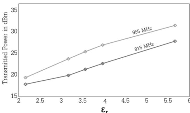
**Figure 3.11.** Minimum tag activation power generated by the reader depending on the permittivity of the tag's support for two frequencies. The tag (see Figure 2.16) is placed on 1 mm-thick dielectric plates with permittivities covering the range 2.2–5.7. The measurement distance between the reader's antenna and tag is 1 m
