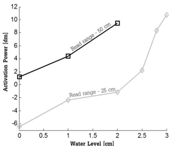
**Figure 3.16.** Measurements of tag activation power (here the power sent by the generator) depending on the water level present in the plastic container. Measurements were taken for two distances between the antenna and the water-filled container
