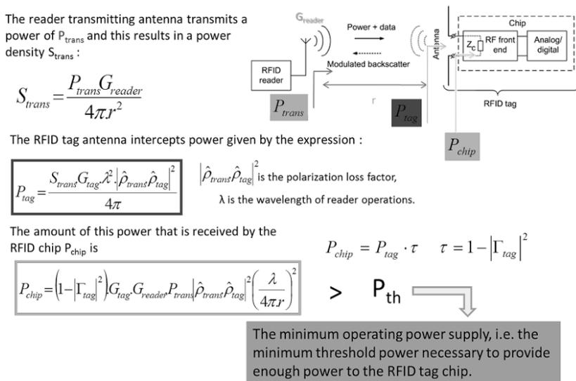
**Figure 3.8.** Power balance applied to an RFID system. Thus, we obtain the expression of power reaching the chip  $P_{chip}$  depending on various parameters such as the coefficient  $\Gamma_{tag}$ . If this power  $P_{chip}$  is greater than the activation power of the chip  $P_{th}$ , the chip has enough energy to function
