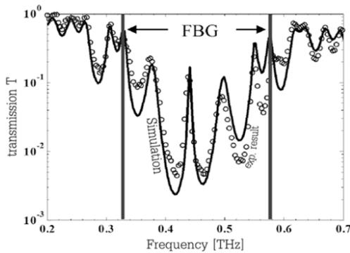
**Figure 5.26.** Simulation and measurement of the transmission coefficient of the PE tag shown in Figure 5.25(a)
