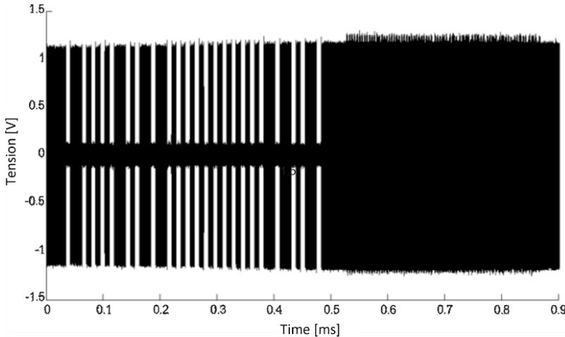
**Figure 2.3.** Oscilloscope measurement of an RFID frame. We can see the reader request (left-hand side) and the tag's response (right-hand side, which is of very low amplitude compared to the reader request)
