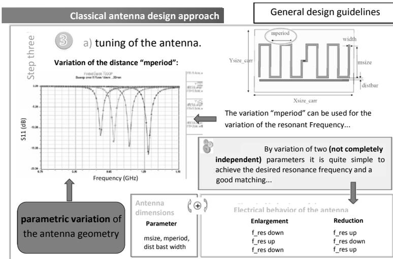
**Figure 2.6.** Illustration of the 3rd stage (antenna tuning) of the classic antenna design method (see Figure 2.5). The idea here is to isolate the key geometric parameters while putting parametric studies in place. The results are represented in the form of abacuses, enabling the linking of the antenna's electrical behavior and its geometry
