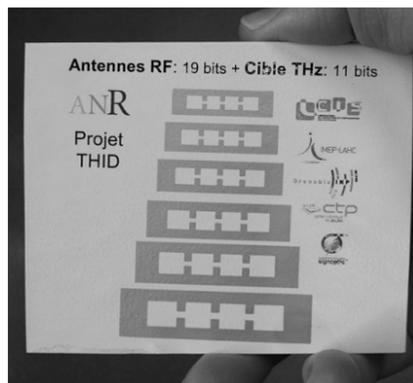
**Figure 5.27.** Photograph of a THID tag, including surface information (RF approach) and volume information (THz approach)
