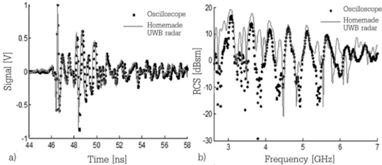
**Figure 5.20.** Comparison between measurements taken with a portable low-cost reader developed on the equivalent-time principle and the acquisition yielded by the 12 GHz oscilloscope operating in real time. a) Temporal signals reflected by the tag shown in Figure 5.4(b), b) RCS obtained without calibration, solely by subtracting the signal from the empty chamber
