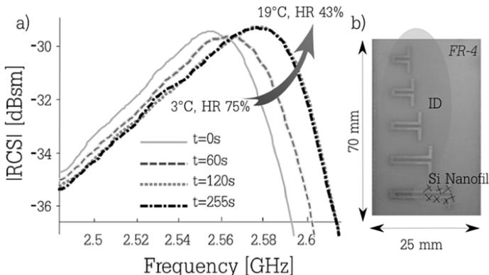
**Figure 6.1.** a) Influence of humidity on the EM response of a resonator containing a deposit of Si nanowire. b) Photograph of a chipless RFID tag integrating the sensor function. For a color version of this figure, see [www.iste.co.uk/perret/radio.zip](http://www.iste.co.uk/perret/radio.zip)
