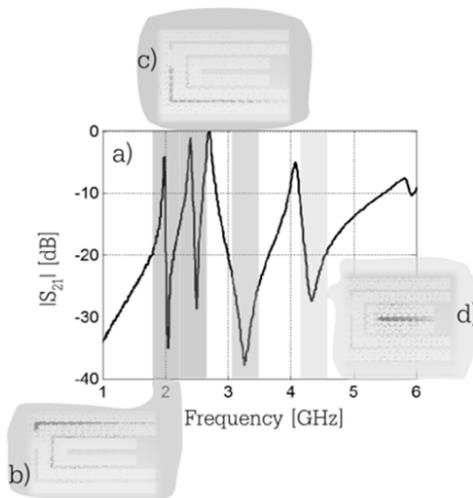
**Figure 4.6.** Illustration of the link that exists between the resonance frequencies and the geometry of C-shaped tags. a) Amplitude of the signal backscattered by the tag according to frequency; the signal is normalized in comparison to the incident signal, b) current density on the tag at a frequency of 2.1 GHz, c) 2.55 GHz and d) 4.4 GHz. For a color version of this figure, see [www.iste.co.uk/perret/radio.zip](http://www.iste.co.uk/perret/radio.zip)
