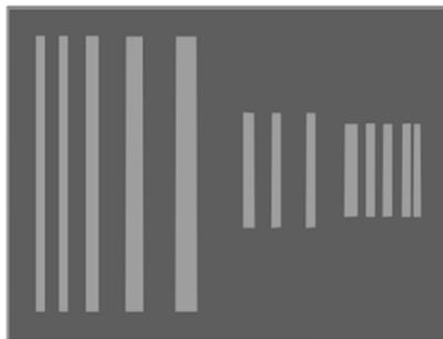
**Figure 5.2.** The first “RF barcodes” introduced in 2005 by Jalaly *et al.* This structure is one of the very first chipless RFID tags with the potential to be compatible with low-cost production and application techniques. Unlike the impression given by the figure above, each dipole has a different length, enabling the coding of one bit
