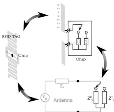
**Figure 2.2.** Equivalent electrical schema of a passive UHF RFID tag
