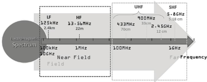
Figure 1.3. Principal frequency bands used by RFID
