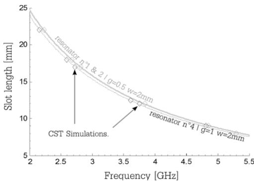
**Figure 4.9.** Variation of slot lengths  $L_s$  according to their resonance frequency. The permittivity is 4.6 and the height of the substrate 0.8 mm. (—) Evolution of  $L_s$  for resonators 1 and 2 with  $g = 0.5$  mm,  $w = 2$  mm. (---) Evolution of  $L_s$  for resonator 4 with  $g = 1$  mm and  $w = 2$  mm. (◇◇◇) CST simulations obtained for specific lengths
