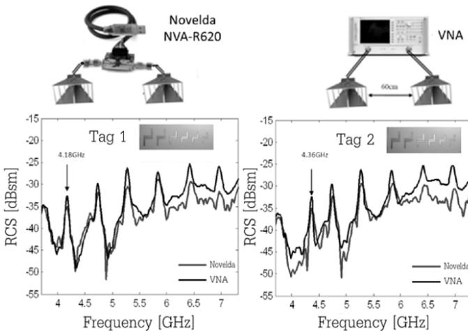
**Figure 5.21.** Comparison between the reference measurement made with a VNA and the one obtained with the Novelda reader for two configurations of the same tag (only the first peak is moved, as expected). For a color version of this figure, see [www.iste.co.uk/perret/radio.zip](http://www.iste.co.uk/perret/radio.zip)
