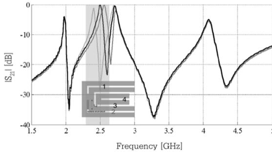
**Figure 4.7.** Illustration of the operating principle of a C-shaped tag. Amplitude of the signal backscattered by the tag according to frequency for three different lengths  $L_2$  of slot no. 2; the signal is normalized in comparison to the incident signal
