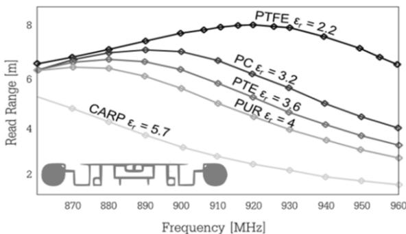
**Figure 2.16.** Simulated read range [2.3] versus the frequency for an antenna created by the automatic design approach to operate in free space. Once the antenna is created (shown at the bottom of the figure), it is simulated in the presence of a dielectric plate (Figure 2.21) whose permittivity is varied between 2.2 and 5.7
