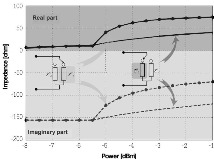
Figure 3.2. Real impedance (solid line) and imaginary impedance (dashed line) of chip NXP GX2L for the high state  $Z_c^1$  (•) and low state  $Z_c^0$  (no marker) depending on the power supplied by the generator for 915 MHz
