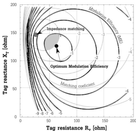
**Figure 3.12.** Graphic representation of tag performance according to the input impedance value  $Z_a$  of its antenna (real part and imaginary part) for NXP chip at 915 MHz. The lines of the  $\tau^0$  (uplink performance) and ME (downlink performance) are traced for different values (in dB). The optimal conditions are represented by points
