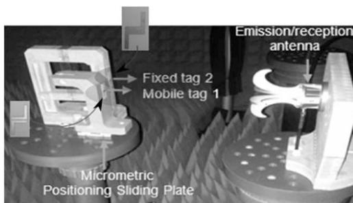
**Figure 6.12.** Measurement bench used in an anechoic chamber for deformation measurement
