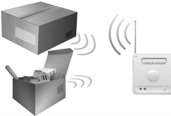
**Figure 4.1.** *Operating principle of a chipless RFID system. The tag is composed of a conductive pattern, possibly printed on a paper or polyethylene terephthalate (PET) substrate*
