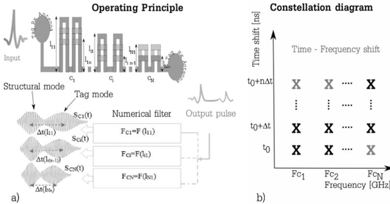
**Figure 5.12.** Temporal illustration of the operating principle of the system based on the use of multiple groups of C-sections. a) Operating principle in a temporal representation. In the illustration, each group is made up of two C-sections. b) Frequency-time constellation diagram, coding principle used. For a color version of this figure, see [www.iste.co.uk/perret/radio.zip](http://www.iste.co.uk/perret/radio.zip)
