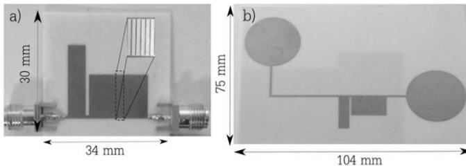
**Figure 5.9.** Example of a structure composed of multiple groups of C-sections; that is, of a line including several groups (2 in this case) of 3 and 10 C-sections, respectively.
