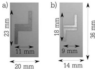
**Figure 6.11.** Photos of the two inverted double-L tags used for the experiment. a) The first one (tag 1) resonates at 4.72 GHz and b) the second (tag 2) resonates at 5.26 GHz
