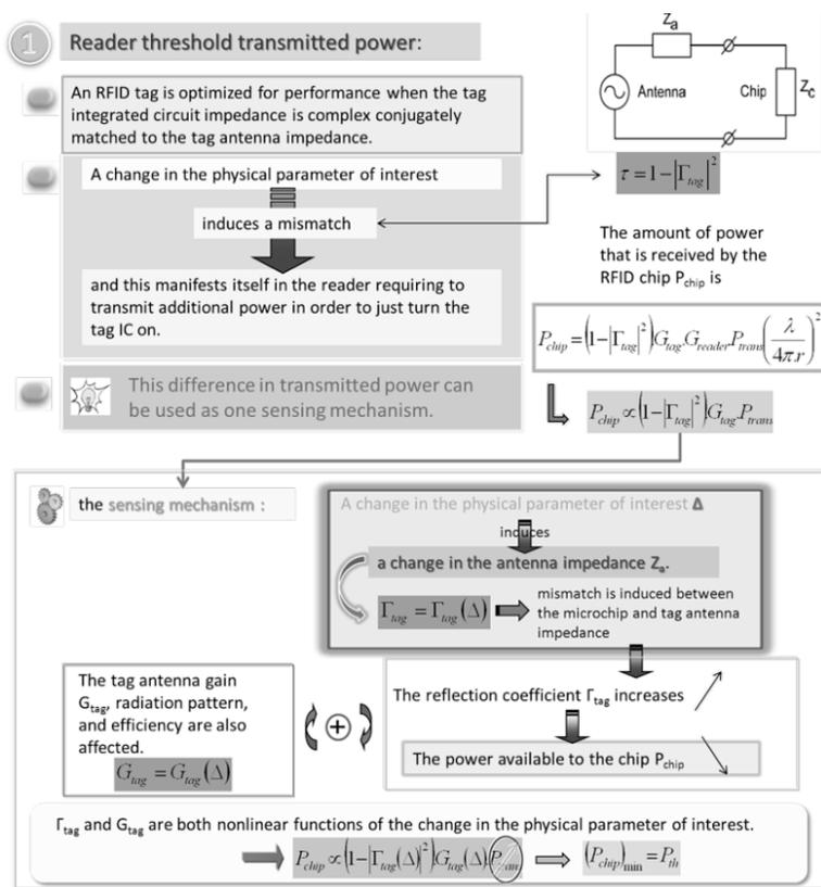
**Figure 3.9.** Operating principle of a sensor based on RFID technology. In this first configuration, the information sought is given by the minimal power transmitted by the reader ( $P_{tran}$ ) enabling the activation of the chip [BHA 10a, PER 11]
