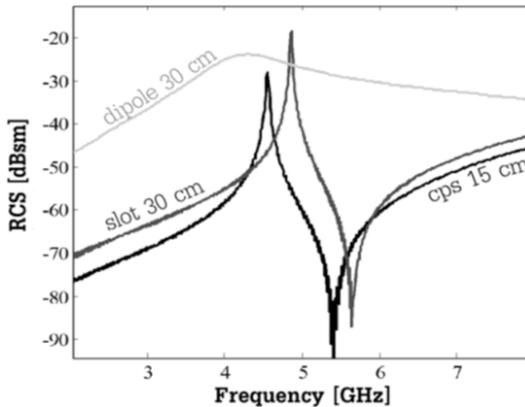
**Figure 4.4.** RCS created by a short-circuited dipole (as in Figure 4.3), a slot (as in Figure 4.3) and a C-shaped structure (as in Figure 4.3(b)). Dimensions:  $\lambda/2=30$  cm,  $W=2$  mm,  $g=0.5$  mm, with no ground plane
