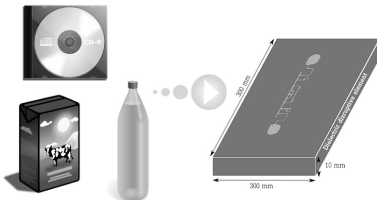
**Figure 2.12.** Taking into account of the environment in the automated design process of robust RFID tags. The EM disruption of the tag induced by a family of products is applied in the simulation by adding to the tag a dielectric plate of variable permittivity and a thickness of 10 mm
