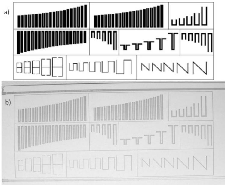
**Figure 5.15.** Examples of printings produced using flexography on paper materials with conductive ink: a) snapshot used containing 10 tags, b) printout obtained. In this example, the total area of the print zone is  $30 \times 10 \text{ cm}^2$
