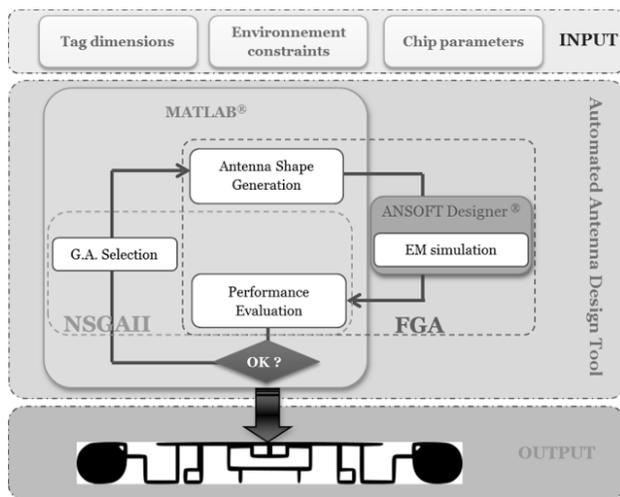
**Figure 2.10.** Theoretical schema of automatic antenna design tool for passive UHF RFID tags
