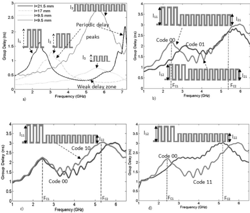
**Figure 5.13.** Principle of the cascading of different groups of C-sections. Group delay depending on frequency for different configurations. a) Simulation of the impact of the length and the number of C-sections on group delay. b) Cascading of two groups, configurations 00 and 01, c) 00 and 10 and d) 00 and 11. Each time, only one of the two lengths varies
