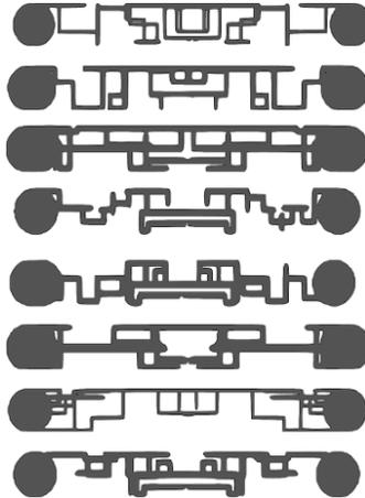
**Figure 2.11.** *Example of antennas obtained using the developed method of entirely automatic passive UHF RFID label design*
