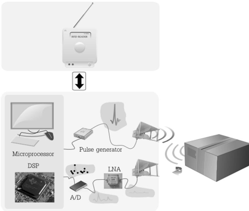
**Figure 5.18.** Operating diagram of a temporal chipless reading system
