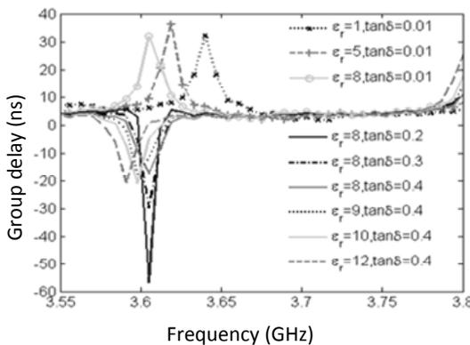
**Figure 6.8.** Simulation of the variation in group delay of the chipless tag-sensor shown in Figure 6.3(a) for different permittivity ( $\epsilon_r$ ) and loss tangent ( $\tan\delta$ ) values. These parameters describe the EM properties of a dielectric box placed on the C-section
