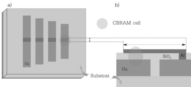
**Figure 6.15.** Reconfigurable chipless tag with three dipole resonators. a) View from above and b) cross-section of the CBRAM cell. For a color version of this figure, see [www.iste.co.uk/perret/radio.zip](http://www.iste.co.uk/perret/radio.zip)
