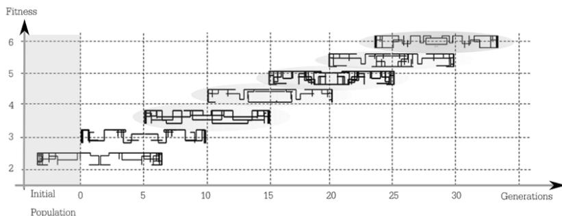
**Figure 2.15.** Evolution of the shape of antennas generated, tested and selected throughout the process of RFID tag design. Only some of the antennas generated are shown. For a selected generation, we are showing the antenna with the best fitness function. The more the number of generations (abscissas) increases, the more the fitness function improves (ordinates)
