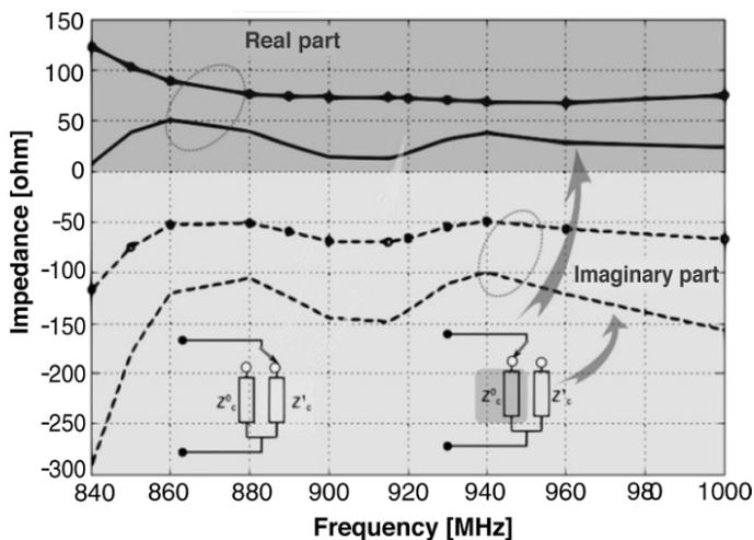
Figure 3.3. Real impedance (solid line) and imaginary impedance (dashed line) of chip NXP for the high state  $Z_c^1$  (•) and low state  $Z_c^0$  (no marker) depending on frequency for a generator power of -2.6 dBm
