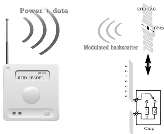
**Figure 2.1.** Schematic diagram of a passive UHF RFID system
