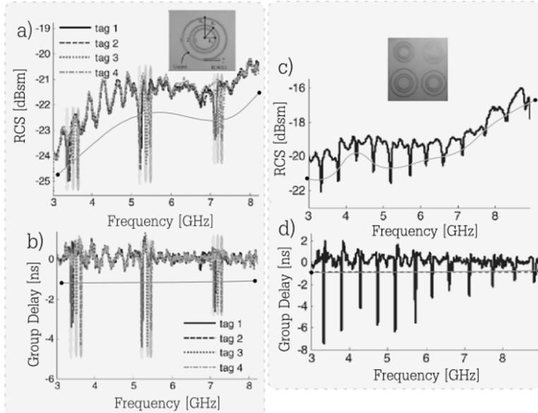
**Figure 5.7.** Results of measurements obtained on invariant tags in relation to polarization. a) and b) RCS and group delay, respectively, of 4 tag configurations containing 3 resonators; c) and d) RCS and group delay, respectively, of tag containing 12 resonators
