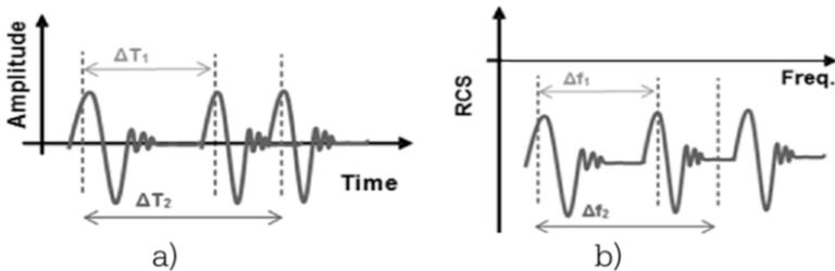
**Figure 4.11.** Decoding principle of an a) temporal and b) frequential tag. Though the tags are intrinsically different, the information they send back can be the same. In this case, the maximas (or minimas) of the signals, expressed in time or frequency, will be used to code the ID of the tag
