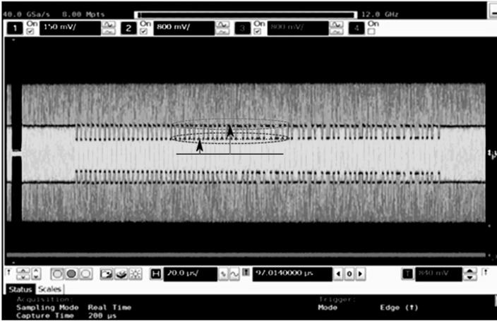
**Figure 3.7.** Capture via oscilloscope of a signal reflected by an RFID tag. The two states (high and low) are clearly identifiable on the frame, making it possible to go back to the values  $E_{scat}(Z_c^1)$ ,  $E_{scat}(Z_c^2)$  (in amplitude and phase). From there, it is possible to obtain the antenna's input impedance using expression [3.16]. For a color version of this figure, see [www.iste.co.uk/perret/radio.zip](http://www.iste.co.uk/perret/radio.zip)
