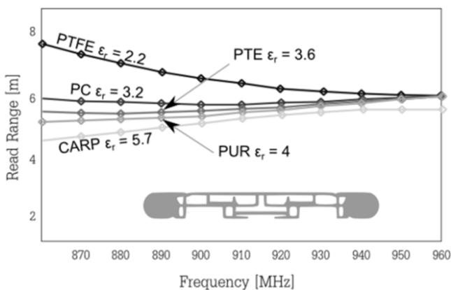
**Figure 2.17.** Simulated read range [2.3] versus the frequency for an antenna produced using the automatic design approach to function on a family of low-permittivity objects (from 2.2 to 5.8). Once the antenna is created (shown at the bottom of the figure), it is simulated in the presence of a dielectric plate (Figure 2.21) whose permittivity is varied between 2.2 and 5.7
