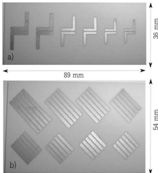
**Figure 5.4.** Photograph of two “depolarizing” tags: a) dual-L resonators and b) shorted dipoles oriented at  $45^\circ$ . These tags operate with a ground plane
