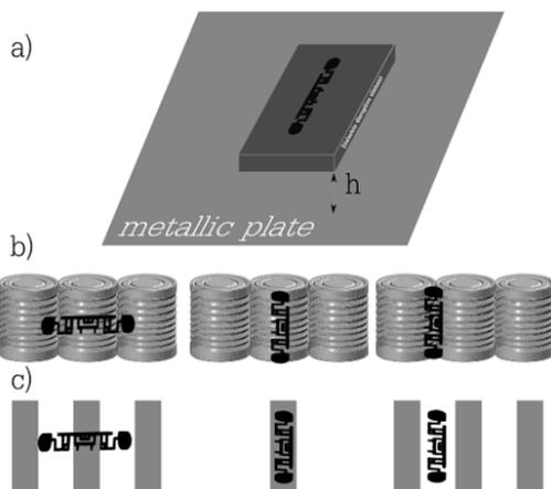
**Figure 2.20.** Model used in Ansoft Designer for the taking into account of a metallic environment. a) Simple model based on the use of a metal plate. b) Real metallic environment studied (here of the metal “can” type –  $h=1-2$  mm). c) Model used to simulate case study b)
