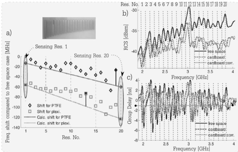
**Figure 5.8.** Result of measurements of 20-bit tag used with the auto-compensation technique. a) Resonance frequency of each resonator for two supports (PTFE and Plexiglas). b)–c) RCS and group delay of a 20 resonator tag: comparison between measurements in free space, on a cardboard box filled with sheets of paper, and obtained via auto-compensation (cardboard corr.) For a color version of this figure, see [www.iste.co.uk/perret/radio.zip](http://www.iste.co.uk/perret/radio.zip)
