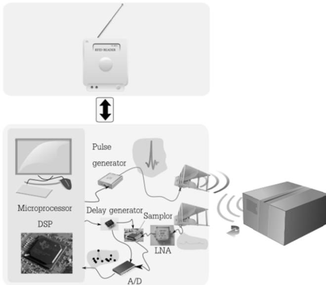
**Figure 5.19.** Operating diagram of a chipless reading system based on an equivalent-time approach
