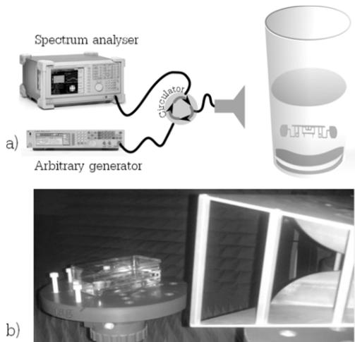
**Figure 3.15.** Measurement bench used to detect the level of liquid in a plastic container using a classic RFID system (tag + reader). The reader is emulated here using an arbitrary waveform generator as well as with a spectrum analyzer.
