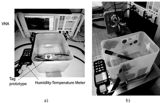
**Figure 6.5.** Test bench used to study the tag's response according to humidity or temperature. a) Measurements in S parameters with a VNA and b) measurements in free space
