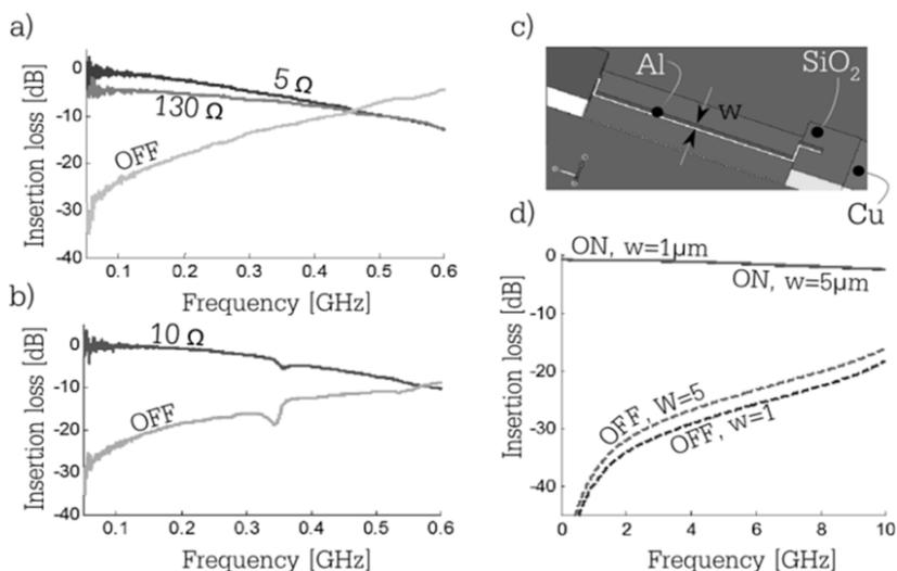
**Figure 6.17.** Insertion losses measured for the sample shown in Figure 6.16(b), with a SiO<sub>2</sub> thickness of a) 160 nm and b) 320 nm. c) Geometry of switch designed to function at up to 10 GHz. d) Simulated insertion losses for the switch presented for several slope lengths  $w$  corresponding to the aluminum electrode. The SiO<sub>2</sub> thickness is 500 nm
