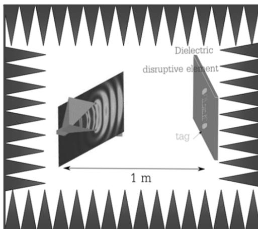
**Figure 2.18.** Measurement bench applied to characterize RFID tags. We measure precisely the minimum power to be sent to cause the tag to function. For a color version of this figure, see <http://www.iste.co.uk/perret/radio.zip>
