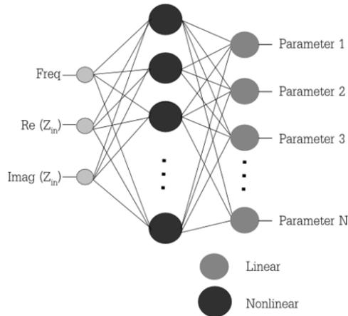
**Figure 2.8.** Example of a neural network used to aid the design of RFID tags
