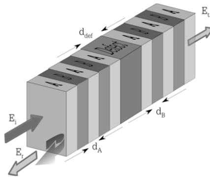
**Figure 5.22.** Operating diagram of a THz chipless tag. The layer labeled “Defect” disturbs the regular alternation of layers A and B, composed by a high and low index material, respectively. Reading is done in transmission in this case. However, for practical reasons, it is possible to add a reflective plane in the center of the structure in order to have reading via reflections, which reduces the tag’s thickness by two
