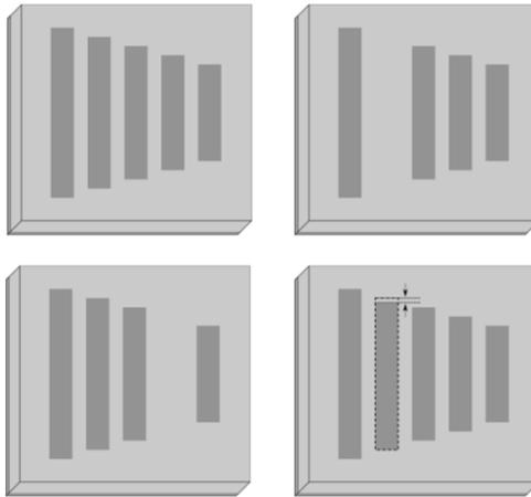
**Figure 4.2.** Example of a chipless dipole tag with a ground plane [JAL 05a].
