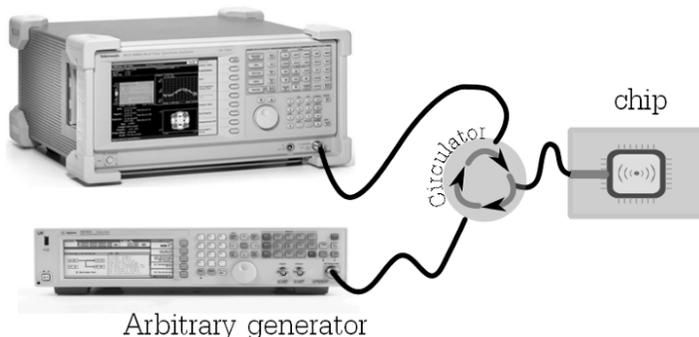
**Figure 3.1.** Measurement bench for RFID chip impedances
