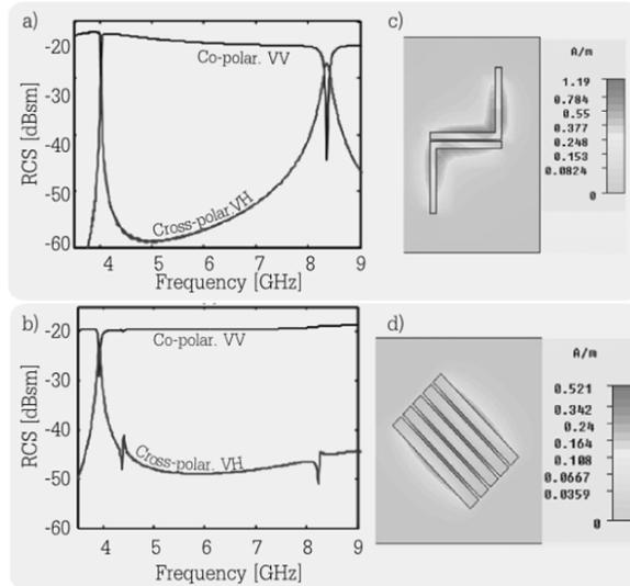
**Figure 5.5.** RCS of coding particles in co-polar (VV) and cross-polarization (VH): a) dual-L resonators, b) shorted dipoles oriented at 45°. c)–d) Surface current density at resonance of the depolarizing coding particles shown in Figure 5.5. For a color version of this figure, see [www.iste.co.uk/perret/radio.zip](http://www.iste.co.uk/perret/radio.zip)
