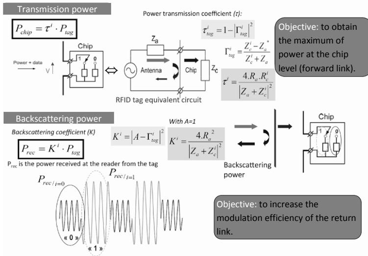
**Figure 2.4.** Schematic and analytical presentation of the values involved in the description of the up- and downlinks of an RFID system
