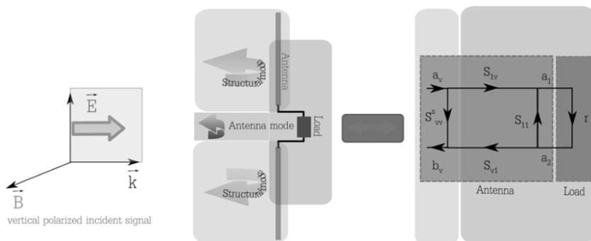
**Figure 3.4.** Model of an antenna in terms of structural mode and antenna mode for excitation in copolarization
