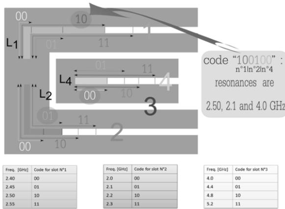
**Figure 4.8.** Illustration of the coding principle via the example of a C-shaped tag. The table of correspondences shows the link between the resonance frequencies of the tag and the associated binary code; here a code on 6 bits. For a color version of this figure, see [www.iste.co.uk/perret/radio.zip](http://www.iste.co.uk/perret/radio.zip)
