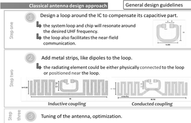
**Figure 2.5.** Illustration of the classic antenna design method for passive UHF RFID tags
