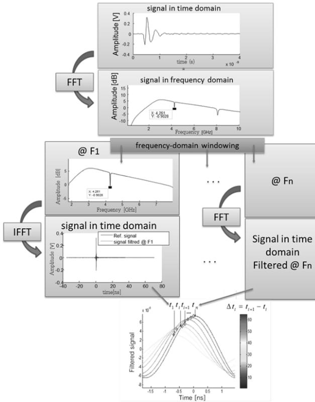
**Figure 6.10.** Descriptive schema of the frequential approach applied to measure a deformation with chipless tags. For a color version of this figure, see [www.iste.co.uk/perret/radio.zip](http://www.iste.co.uk/perret/radio.zip)
