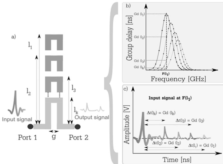
**Figure 5.10.** Operating principle of a tag based on the use of a C-section. a) schema of a C-section whose length  $l_i$  is variable. b) Group delay depending on frequency for different line lengths  $l_i$ . c) Correspondence in the temporal domain at frequency  $F(l_1)$ . For a color version of this figure, see [www.iste.co.uk/perret/radio.zip](http://www.iste.co.uk/perret/radio.zip)
