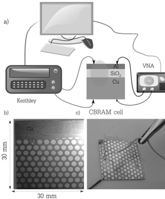
**Figure 6.16.** *a) Operating schema of DC and RF measurement. b) Photograph of samples produced, with each aluminum disk corresponding to an RF switch, that is, to an MIM stack. c) View of the measurement bench used to measure the transmission coefficients of the switch using a VNA*
