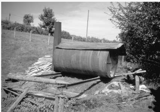
A mobile retort kiln, set up for easy unloading: the chimney is removed, the drum is rolled along the rails, and the charcoal falls out.
