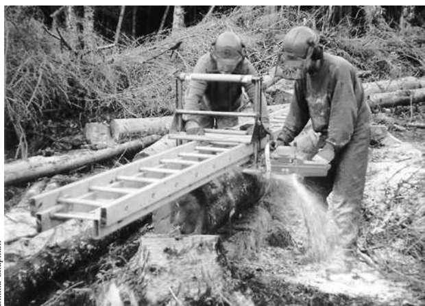
David and Rob Blair using the portable mill they made from a chainsaw and a ladder.
