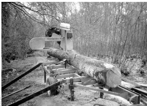
The Wood Miser, a top-of-the-range mobile sawmill.
