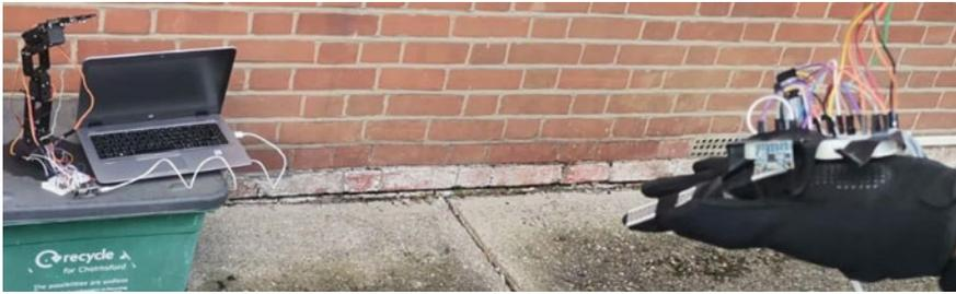
Fig. 30 Transmitter and receiver systems showing different angles of gestures
