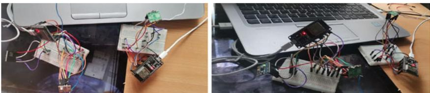
**Fig. 23** Breadboard simulation of the LoRa (transmitter and receiver) interfaced with mpu6050 accelerometer and gyroscope
