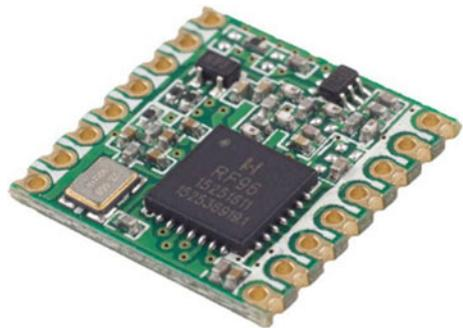
**Fig. 2** Typical components in a LoRa transceiver chip [32]
