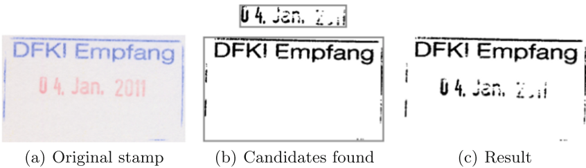
Fig. 7. A two-color stamp is split into two segments during the process and then merged again on output of the stamp detection algorithm.
