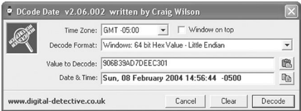
FIGURE 17.7 DCode used to convert 64-bit FILETIME date-time stamps from their hexadecimal representation.
