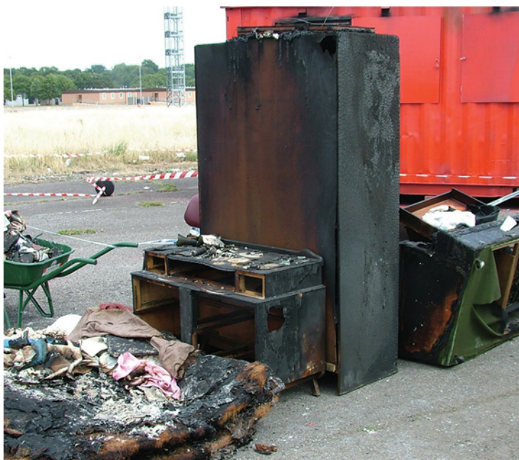
Figure 12.2 Wreckage of a 'suspicious fire' being investigated as part of the NTC Fire Investigation Training Course. Perhaps the most ambitious of dynamic and immersive programmes, the Fire Investigation Course centred on the real-time investigation of simulated fire scenes set out in ISO containers.
