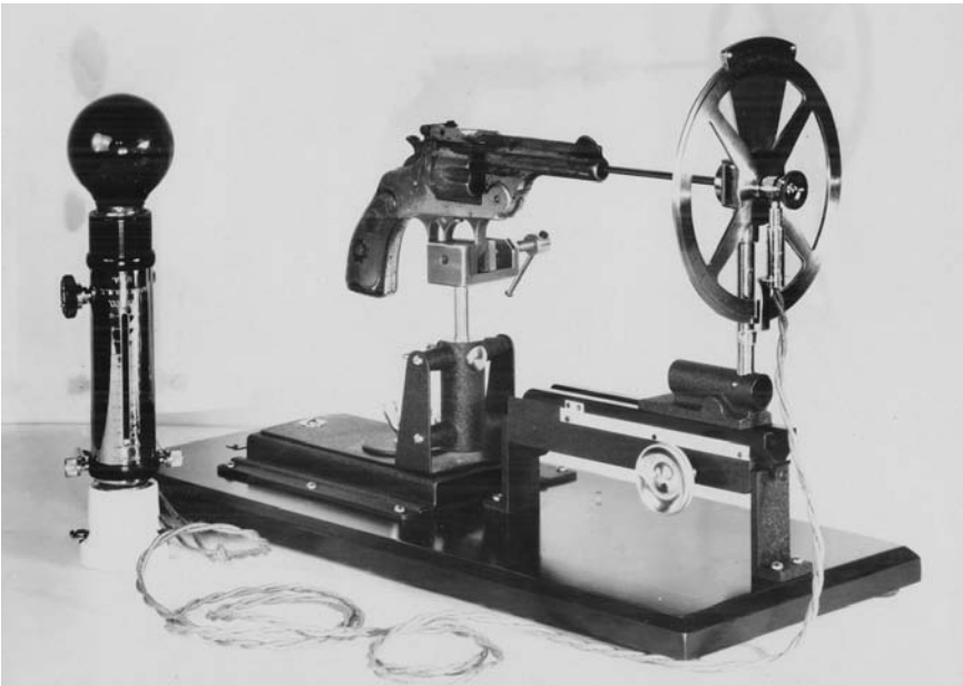
The helixometer was invented by physicist John H. Fisher around 1923. The helixometer is a long, hollow probe with an attached light and magnifying glass that could be used to look into a gun barrel and examine the twist, or helix, of its rifling. The helixometer shown here, called a Spencer helixometer, was used at Calvin Goddard's Scientific Crime Detection Laboratory at Northwestern University. (Northwestern University Archives)
