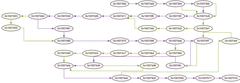
Fig. 4. A behavior graph that presents how Microsoft notepad.exe works. Different colors mean the different execution paths.
