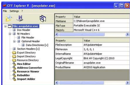
Figure 5.27 Parsing a suspect PE file with CFF Explorer
