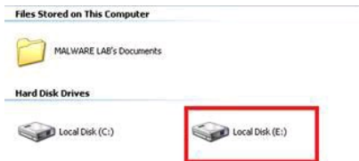
Figure 1.29 Remote subject system hard drive through F-Response
