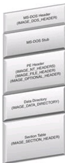
Figure 5.26 The Portable Executable (PE) file format
