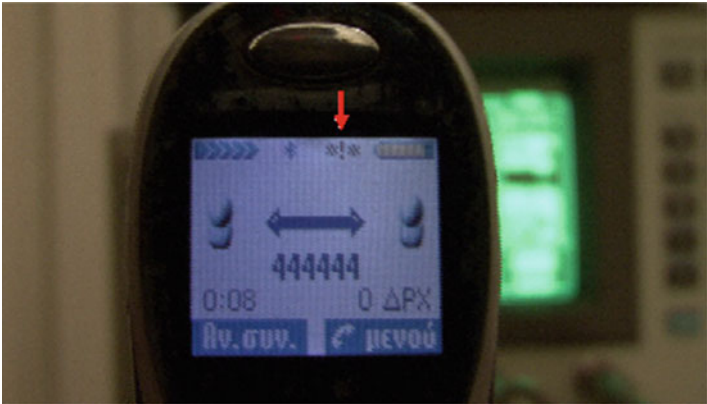
Fig. 3.8 Stars with the exclamation mark in the middle indicate (to a savvy user) the lack of encryption
