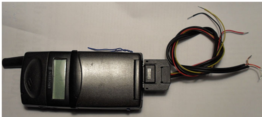
Fig. 6.1 Mobile phone-detonator. We have a clear view of the connection with the mobile phone using the input/output port
