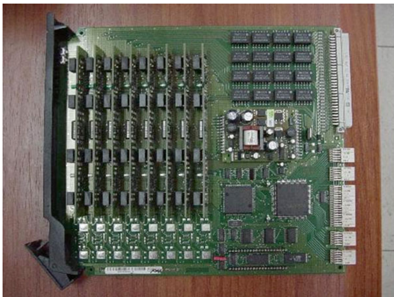
Fig. 3.11 A PBX board serving 32 digital sets
