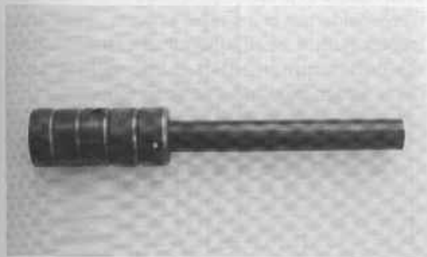
PHOTO 17: Barrel fully assembled with all collars fitted.
