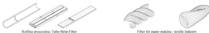
Fig. 1.22 Technical process diagram of bamboo fiber. Source Redrawn according to the related technical patents
