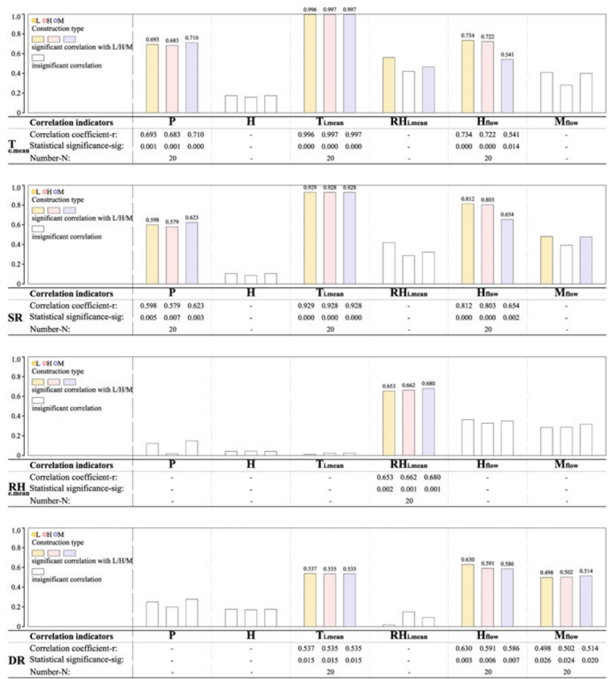
Fig. 2.10 HAM model group correlation analyses between meteorologic parameters (annual average exterior air temperature T_{e,mean} , annual total solar radiation SR, annual average exterior relative humidity RH_{e,mean} , and annual total driving rain DR) and the simulation results (Group 1 annual total/mean values)
