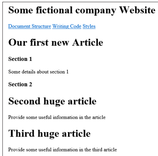
FIGURE 1-6 Using the <section> element within an <article> element
