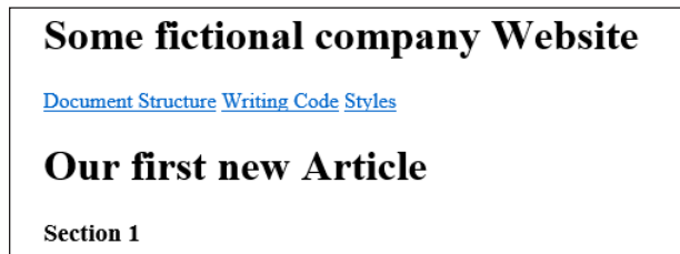
FIGURE 1-3 A navigation menu created using the <nav> element
