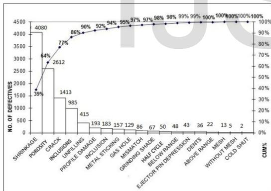
Figure 7 Pareto chart of rejections of Al alloy wheels for one year
