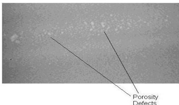
Figure 6 Porosity defect on Al alloy cast wheel [11]
