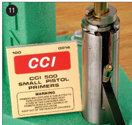
11. Pick the appropriate primer from the listing in any loading manual. In this case, CCI 500 Small Pistol primers are correct for the .38 Special cartridge.
