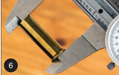
6. After cleaning (if a case lube was used), check each case for the proper overall length. This is easily done on a dial micrometer or the inexpensive plastic gauges sold by many of the loading manufacturers.
