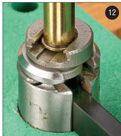
12. Seat primers carefully. One method is on the press, as shown, with the attached primer arm. Another is to use a hand-priming tool, and a third would be a special automatic priming tool. Make sure the primer is fully seated to the bottom of the pocket.
