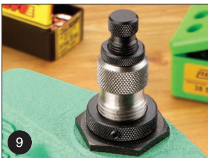
9. Replace the sizer die with the neck expander (second die in the set) setting the case flare to accommodate the bullet base. Do not over flare the case mouth.
