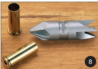
8. After trimming, where necessary, a deburring tool is used to clean up the case mouth. Using the pointed end creates a slight chamfer in the case mouth; the opposite end is for the outside edge.
