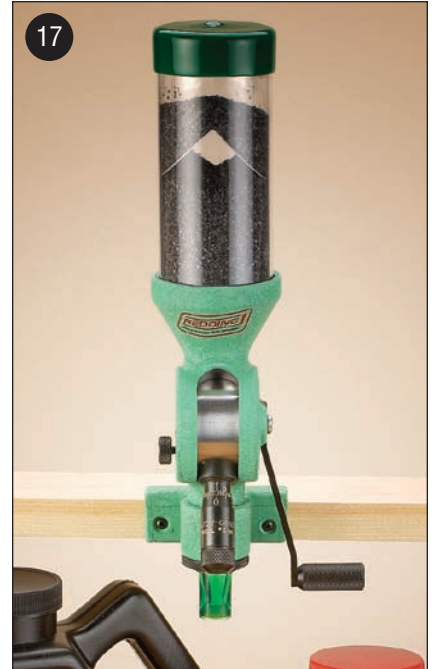
17. Now is the time to set up the powder measure on a rigid surface or use the screw clamps some companies offer.
