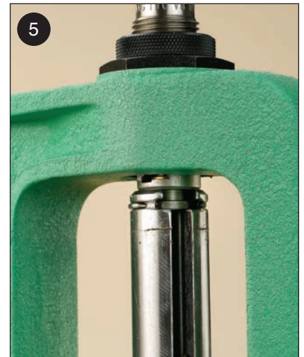
5. Run all the cases all the way up and into the sizing die. If a fired case is used, the primer will be expelled at this time also.
