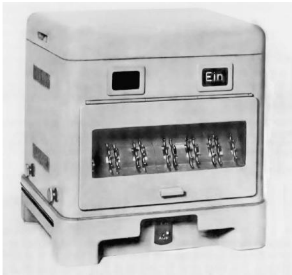
Figure 8.3. Tunny. When attached to a teletypewriter/teleprinter, the Tunny machine encrypted the text that the operator typed at the keyboard. The rims of the Tunny's encoding wheels are visible behind the see-through panel. Picture Library, Imperial War Museum, London. Photograph restored by Jack Copeland and Dustin Barrett. Reproduced with permission.
