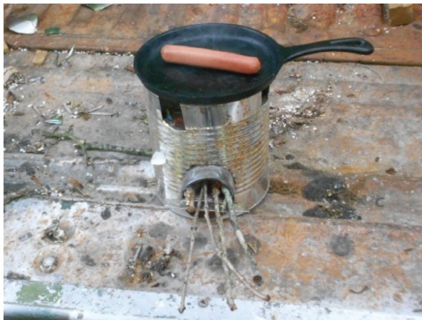
Figure 41.1 Finished rocket stove
