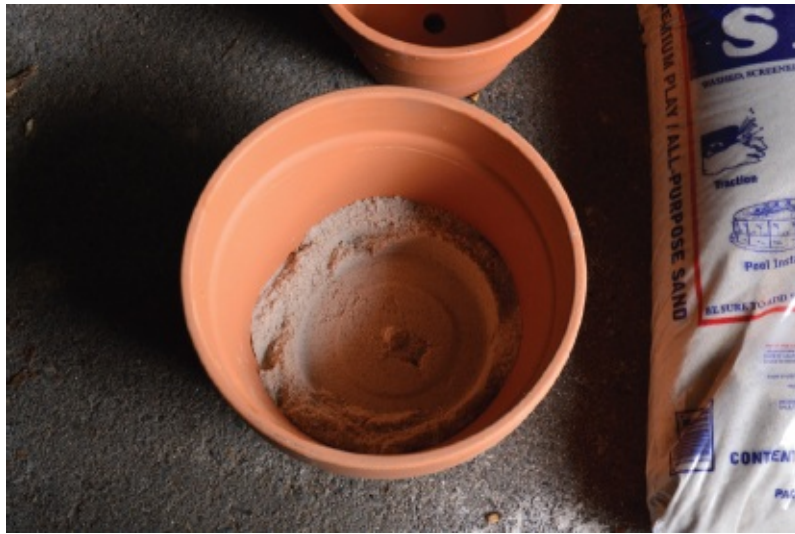
Figure 46.3 Fill bottom with enough sand so that the smaller pot will fit flush with the top of the outer pot.
