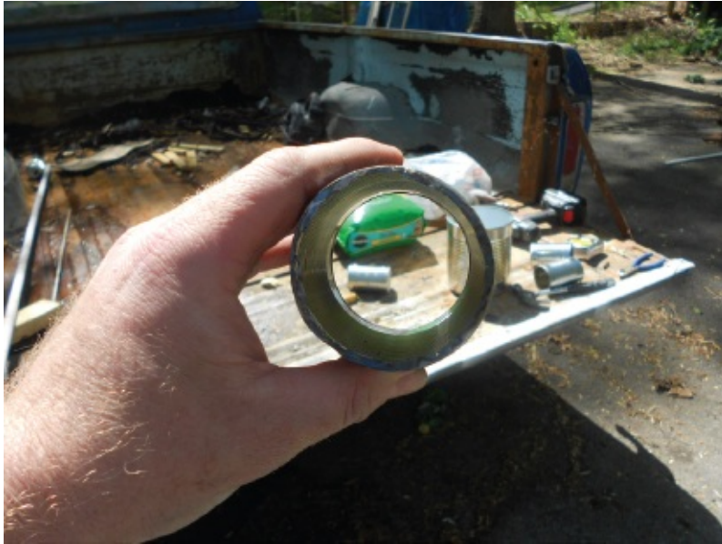
Figure 41.6 Bottom is cut out of soup can B.
