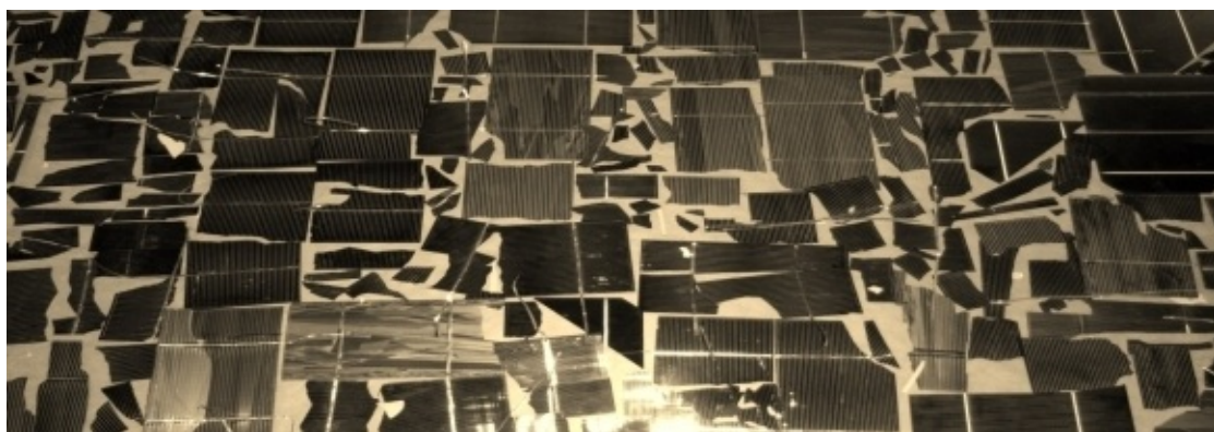
FIGURE 1.1 This is a collection of broken cells from a decade of handcrafting solar panels, and while it may seem daunting, it is just part of the territory when practicing this trade. The goal here is to learn from my mistakes so you don't end up with a collection such as this. If you DO happen to break solar cells, it is not a problem, you will get the feel for how to handle them in short order, but it will save you lots of grief by paying heed to my warnings about securing your work areas.
