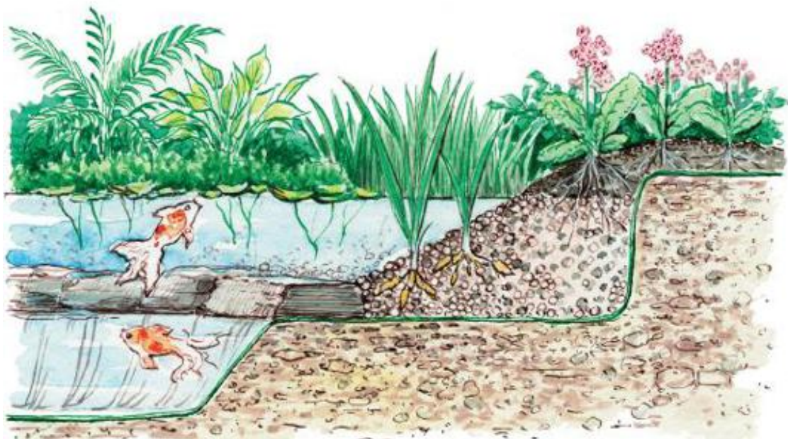
This pond edge, based on a design by Earle Barnhart of Great Work, Inc., allows animals and birds access to the water. At the same time, the gravel beach looks far more natural than ponds edged with rocks, a pattern rarely seen in nature.
